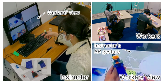
Figure 1: One-to-many AR remote collaboration system used in this study.
